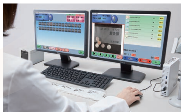
Judgment result list and detailed image of each pouch can be checked at the same time on 2 monitors.
